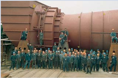
Induced draught fan for Tuoketuo power station on test in Howden Hua's factory in China.
