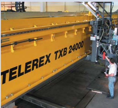
One of two ESAB TXB fully automatic cutting machines for steel panels up to 30 mm thick ordered by Spain's largest shipyard in September
