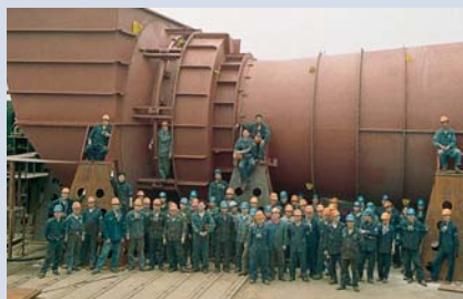
Induced draught fan for Tuoketuo power station on test in Howden Hua's factory in China.
