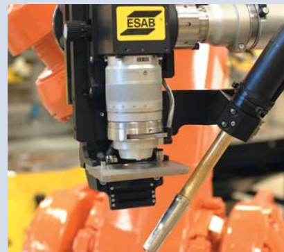
ESAB laser-hybrid welding head for robot applications. This technology is finding growing potential within the automotive sector.
