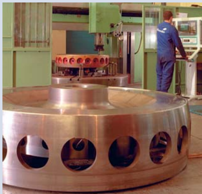
Axial flow fan hubs in Howden Power's Belfast machine shop.
