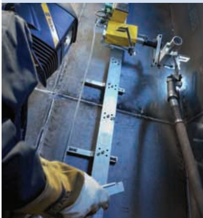
The ESAB "railtrac" automated welding system for shipbuilding and other large applications
