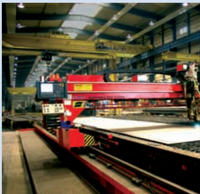
ESAB Suprarex oxy-fuel cutting machine with variable bevel angle capability in a heavy steel fabrication mill
