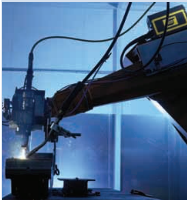
Laser-hybrid welding for robot applications at the ESAB process centre in Gothenburg
