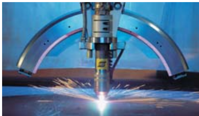
Plasma cutting Bevelhead, manufactured by ESAB
