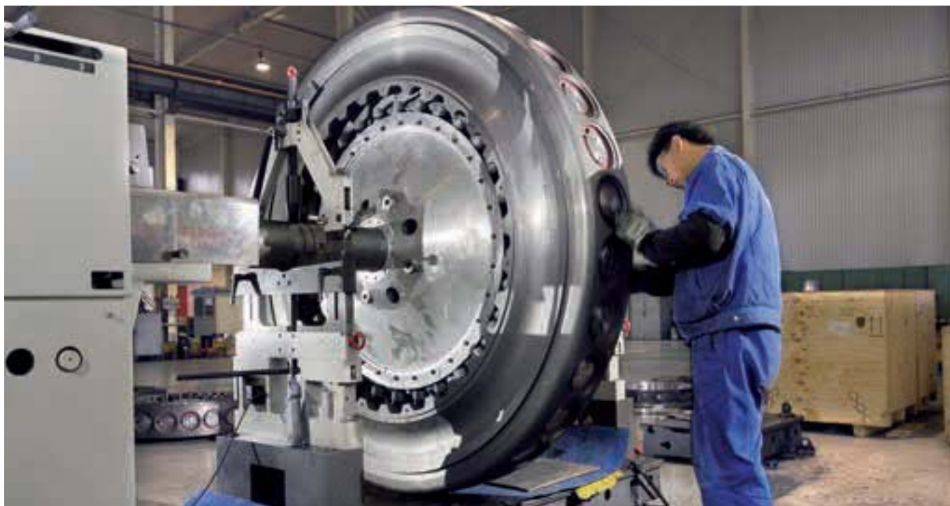
Axial flow fan hub undergoing balancing in the Howden Hua facility in Weihai, China
